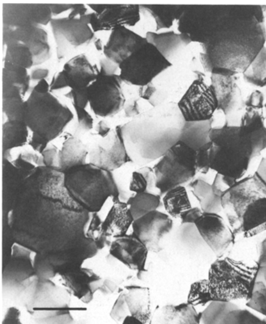
Figure 1 Typical microstructure of Material B; TEM micrograph. Scale bar = 1 \mu\text{m} .
